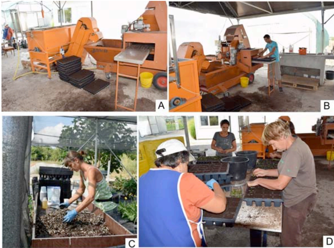
Fig. 3. A, B: machine for mixing the substrates for acclimatization and another machine for dispensing the substrates into cell trays at IndPI, C: preparing a small batch of substrate for the ex vitro acclimatization test, D: ex vitro transfer of walnut plantlets into cell trays with substrate
